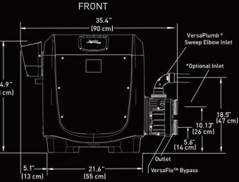
NOTE: Dimensions are identical on all heater models
