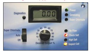
NOTE: Check Salt & Inspect Cell LED's will also be ON if the control is set for the wrong Turbo Cell type or the cell is unplugged.
