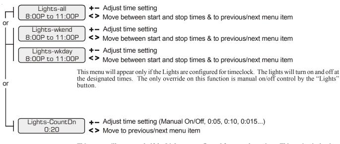
This menu will appear only if the Lights are configured for countdown timer. This setting is the time after you manually turn on the lights until the Pro Logic automatically turns off the lights. You can also manually turn off the lights at an earlier time by pressing the LIGHTS button.
