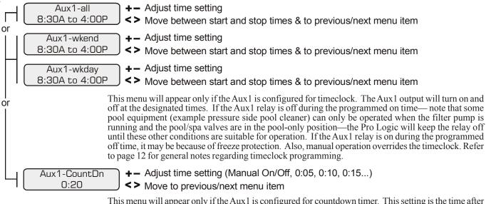
This menu will appear only if the Aux1 is configured for countdown timer. This setting is the time after you manually turn on the Aux1 relay until the Pro Logic automatically turns off the relay. You can also manually turn off the relay at an earlier time by pressing the AUX1 button.
