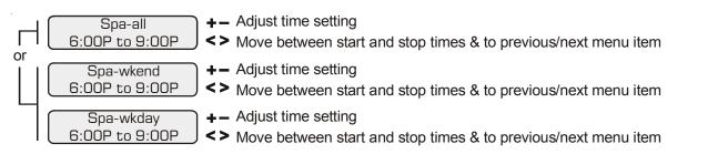
This menu is only available if the system has been setup for "pool and spa-std". During the programmed spa time, the Pro Logic will move the pool/spa valves into the "spa-only" position and turn on the filter pump. The heater will automatically heat the spa up to the programmed spa temperature. This programmed spa operation will take precedence over all other automatic functions, only manual operation of the filter button or pool/spa valve button will override this function.
