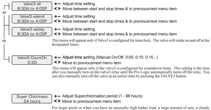
For larger pools or when you have an unusually high bather load, a large amount of rain, a cloudy water condition, or any other condition that requires a large amount of chlorine to be introduced to the pool, may require more hours of Superchlorination. Smaller pools require less hours of Superchlorination.
