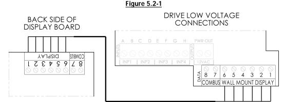
**Note:** Connection wire must be rated for a minimum of 300V, and may be up to 500 feet in length. Use removable 6-position terminal block connectors for wiring connection to display and motor drive board taking care to note the wire colors and corresponding numbers next to the connectors. Do **not** connect to the upper input terminals shown as light gray above.
