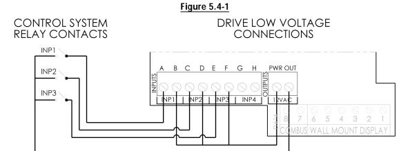
Connection wire must be rated for a minimum of 300V. See section 6.6.11 for more details. Do **not** connect to the lower "COMBUS" or wall mount "DISPLAY" data terminals.
