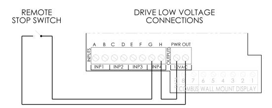
**Note:** Connection wire must be rated for a minimum of 300V. Switch must be latching type; pump is stopped when circuit is closed.
