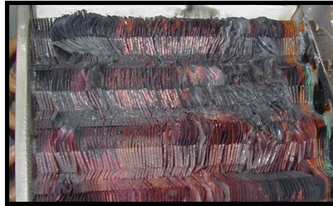
Annealed fins – Low Water Flow
